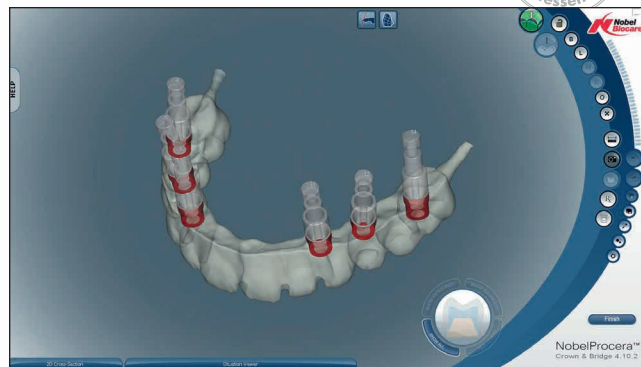
Fig 14a Scanned framework prototype in the design module of the Procera System.
