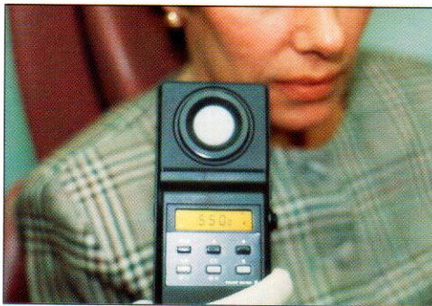
Fig 2 Color temperature meter is used to check the lighting conditions around the patient's face.
