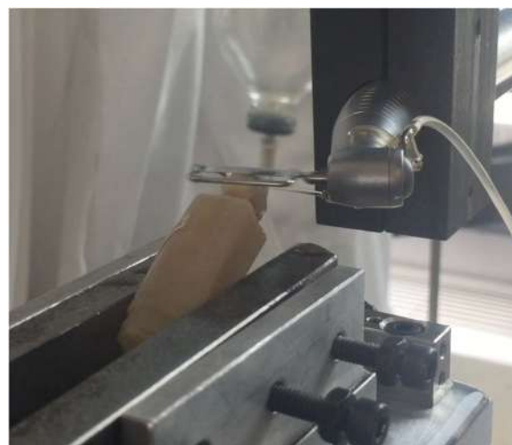
Fig. 1 Oscillating diamond strip and contra-angle adapted on the Instron Universal Testing Machine for the experimental analysis
