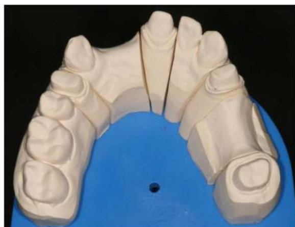
Fig. 7 Finalized sectioned cast. Two scanings followed: first, the sectioned casts were digitized with the reference scanner. Second, they were digitized with the desktop scanner
