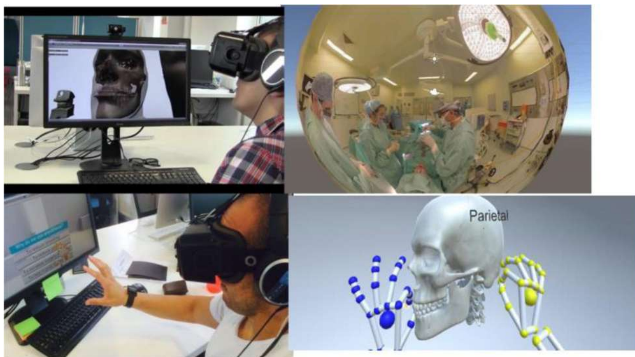
Fig. 2 Oculus Rift showing 3D digital data, the operating theatre, the leap motion sensor tracks the trainee's hands to select items from the menu or apply a surgical instrument (PhD thesis of Yeshwanth Pulijala The University of Huddersfield, 2017)
