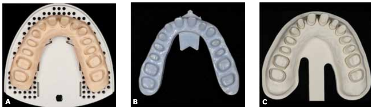
Figure 1. Computer-aided design/computer-aided manufacturing-generated casts. A. Stereolithographic cast based on data from CEREC AC with Bluecam (Sirona, Bensheim, Germany). B. Stereolithographic cast based on data from Lava Chairside Oral Scanner C.O.S. (3M ESPE, St. Paul, Minn.). C. Milled cast based on data from iTero (Align Technology, San Jose, Calif.).
