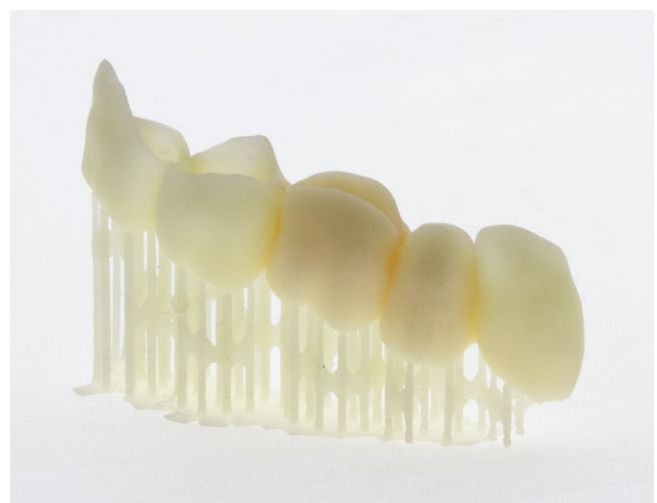
FIGURE 3 Additively manufactured interim dental restoration before the removal of the supportive structures
