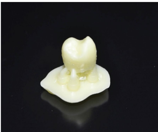
Fig. 9 – Example of 3D printed crown before polishing and removal of supports.
