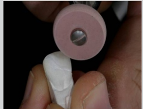
Fig 11. The rubber wheel is used to finish the texture and to thin out the margins without chipping it.
