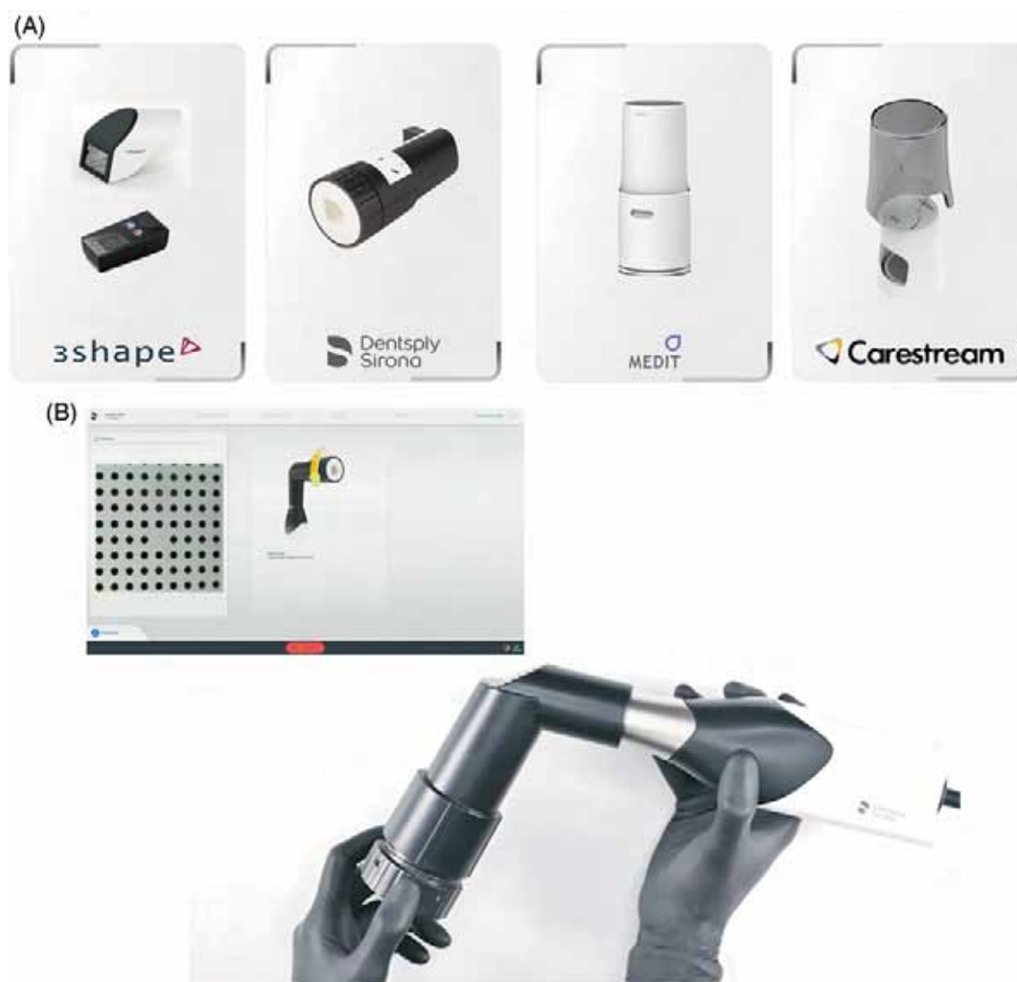
FIGURE 4 (A) Examples of calibration devices provided by IOS's manufacturers for calibrating their systems. (B) Representative calibration protocol for an IOS (PrimeScan; Dentsply Sirona). IOS, intraoral scanner.
