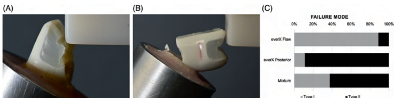
FIGURE 5 Failure modes (A, type I restorable, B, type II non restorable) and distribution for each group (C).
