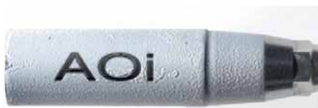
FIGURE 7 Nonhomogeneous coating distribution. This may cause improper alignment when using the best fit function in the CAD software
