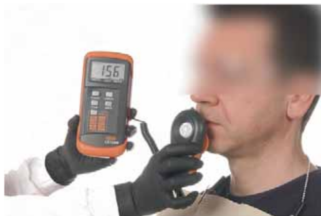
FIGURE 6 Ambient light intensity should be measured at the patient's mouth by using a luxmeter.
