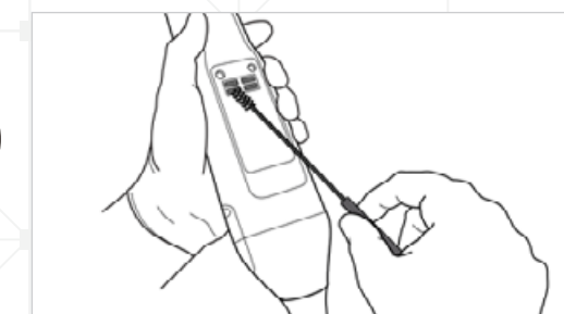
Figure 4: Remove marks and stains using a soft bristle brush
