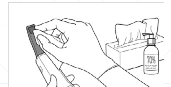
Figure 5: Wipe the optical surface of the wand with IPA
